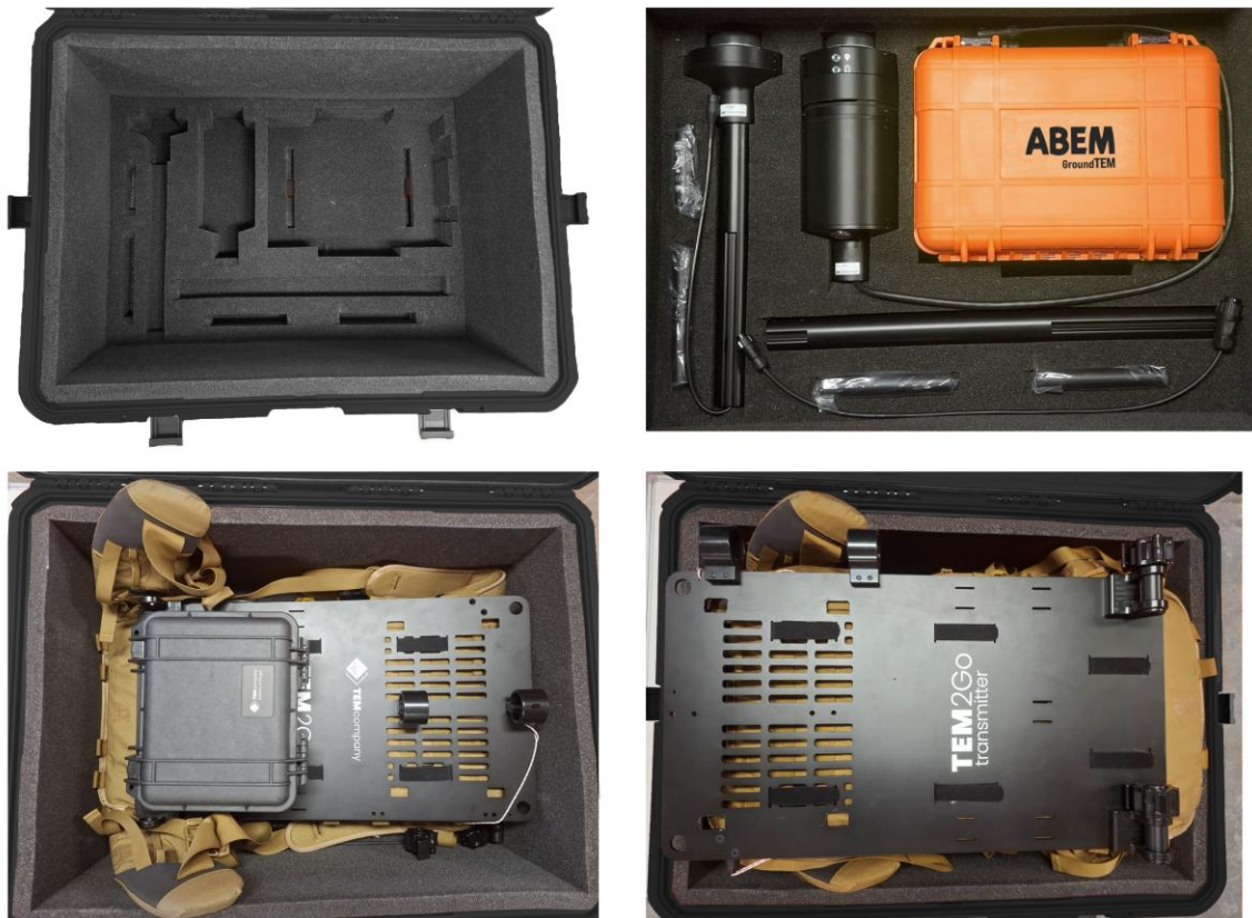
Figure 27: Packing components in the hard case. Start by packing the smaller components in the designated slots in the foam (up). Next pack the two backpack plates, with the battery charging suitcase located between them (down).
