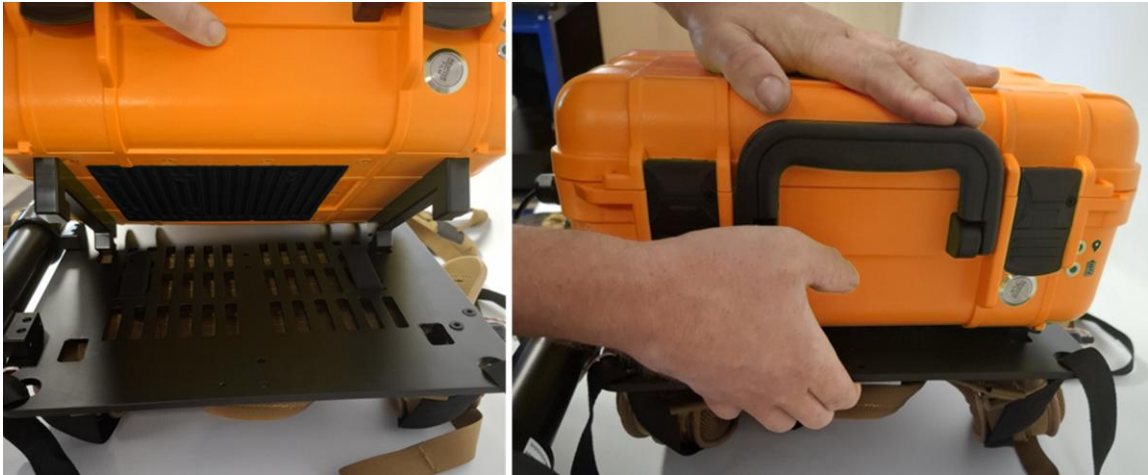
Figure 20: How to mount the Tx unit onto the transmitter backpack.
