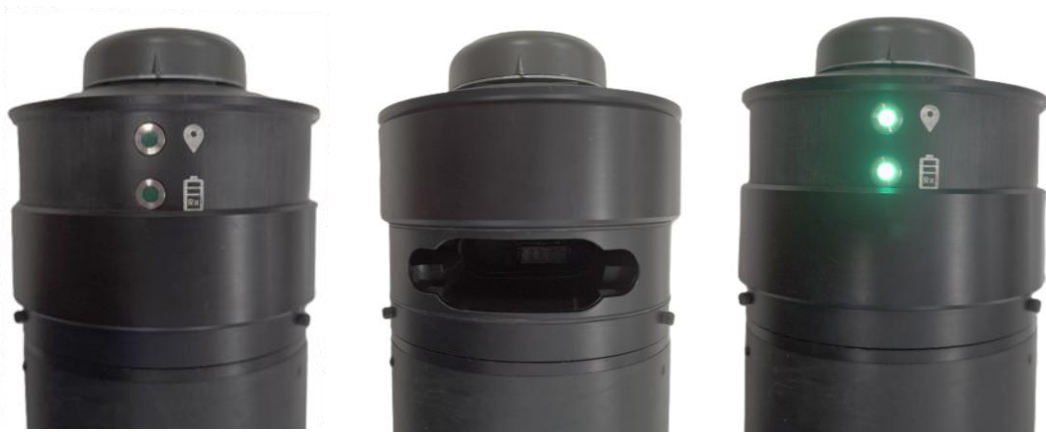
Figure 8: Steps to power the receiver unit. After inserting the battery and pressing the power button, the two LED lights turn on.
