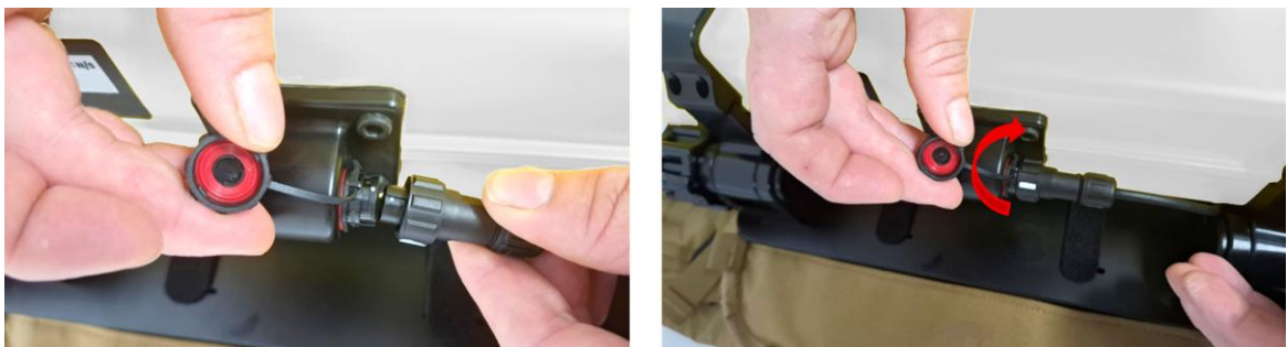
Figure 23: How to connect the Tx unit cable to the connector on the Tx coil.
