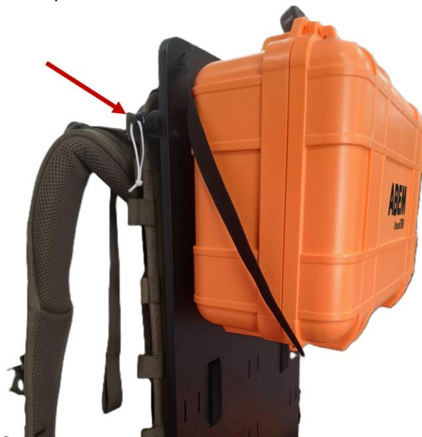
Figure 25: Pull safety pin to release and dismount the GroundTEM Trek unit from the backpack.
